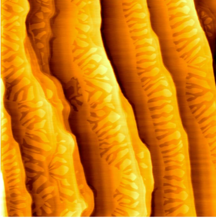
FIG. 1. (Color online) Atomic force microscope image from Ref. 12 of a SiC(0001) surface graphitized at T \sim 1600 °C in an induction furnace with a background Si pressure P \sim 1 \times 10^{-5} torr. The field of view is 10 \mu\text{m} . The steps descend from left to right.
